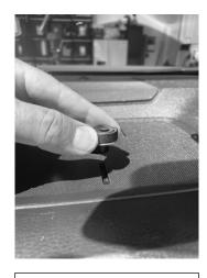
Line up the screw with the hole you previously drilled.
