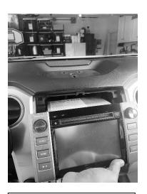
With your handle supporting the bottom of the radio, carefully pull it all the way out.
