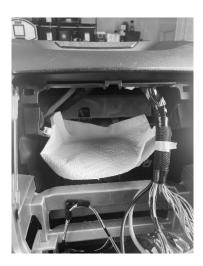
Place a paper towel in the void to catch any debris from cutting or drilling.
