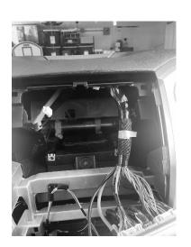
Make sure the cables are clear underneath the dash so they do not get cut or damaged.
