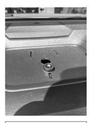
This is the placement of the magnetic and repeat on the other two slots. (Disregard the 3/4" hole in pic. This is drills for hidden cables).
