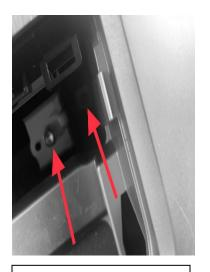
Carefully remove the two 10mm bolts on the right holding the radio.
