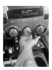
With your fingers underneath the panel pull the climate control panel straight forward.
