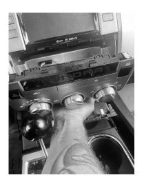
Disconnect this cable and remove the climate control panel or let it stay in place.
