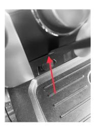
Insert a pry tool here above the 12v outlet and gently pull the edge out.
