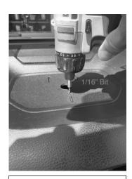
With a 1/16" drill bit, carefully drill a small hole at the tops of each of the three slot that hold the dash mat in place. Just drill enough to penetrate the plastic, do not drill the full length of the bit!!
