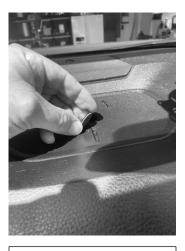
With the dash mat removed place the magnet at the top of the three grooves that hold the dash mat in place.
