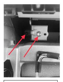
Carefully remove the two 10mm bolts on the left holding the radio.
