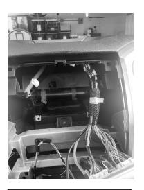
Clear away any cables right underneath the dash so they do not get cut or damaged. Now take the three wing nuts and tighten them to the machine screws. Do not over tighten.
