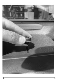
With the machine screw placed inside the magnet line up the screw with the hole you previously drilled.
