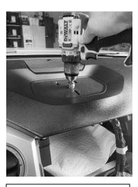
Drill a 3/4" hole in the center of the three divots. All the cable from your devices should fit through this hole.
