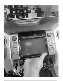
With your fingers underneath the radio pull the radio straight forward.
