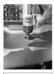
With a 9/64" drill bit, carefully drill a small hole at the tops of each of the three slot that hold the dash mat in place. Just drill enough to penetrate the plastic, do not drill the full length of the bit!!
